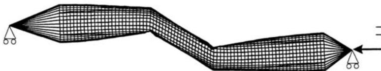
FIGURE 42.16 FE model of bridging pipe. (Source: Venart and Tan, 2000.)
