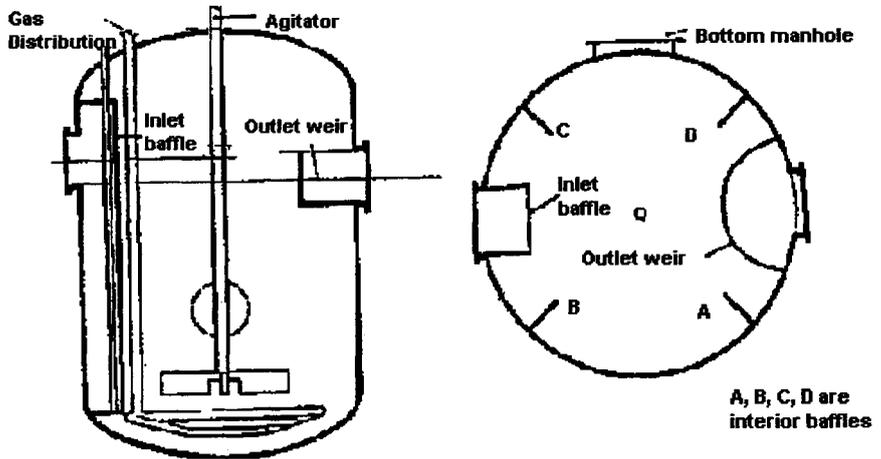
FIGURE 42.3 Reactor vessel details; elevation and plan views. (Source: Artingstall, 1974.)
