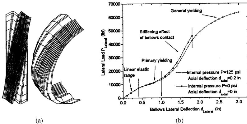
FIGURE 42.11 Large-scale deformation of bellows: (a) with imposed axial deflection under internal pressure and lateral loading; (b) load in lb<sub>f</sub>, pressures in psig, deflections in inches.
