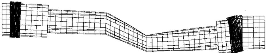
**FIGURE 42.18** FE model of the Flixborough bypass assembly at an internal pressure of 0.964 MPa (125 psig); deformation scale exaggeration is 100. (Source: Venart and Tan, 2000.)
