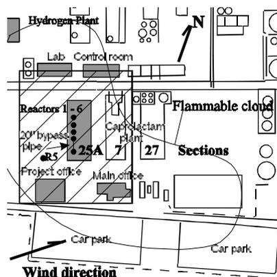
FIGURE 42.2 Portion of the Nypro site plan showing section 25A and the reactor train.
