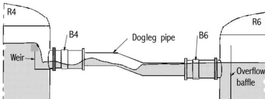
**FIGURE 42.5** Reactor train vessels R4 to R6 with the temporary bypass pipe with the liquid levels as for full flow. (Source: Teng-yang et al., 2000.)
