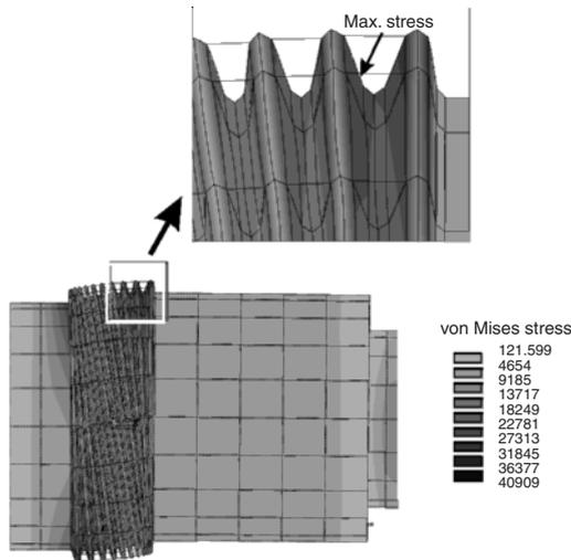
**FIGURE 42.19** Static equivalent (von Mises) stress upper B4 bellows, stress in psi.
