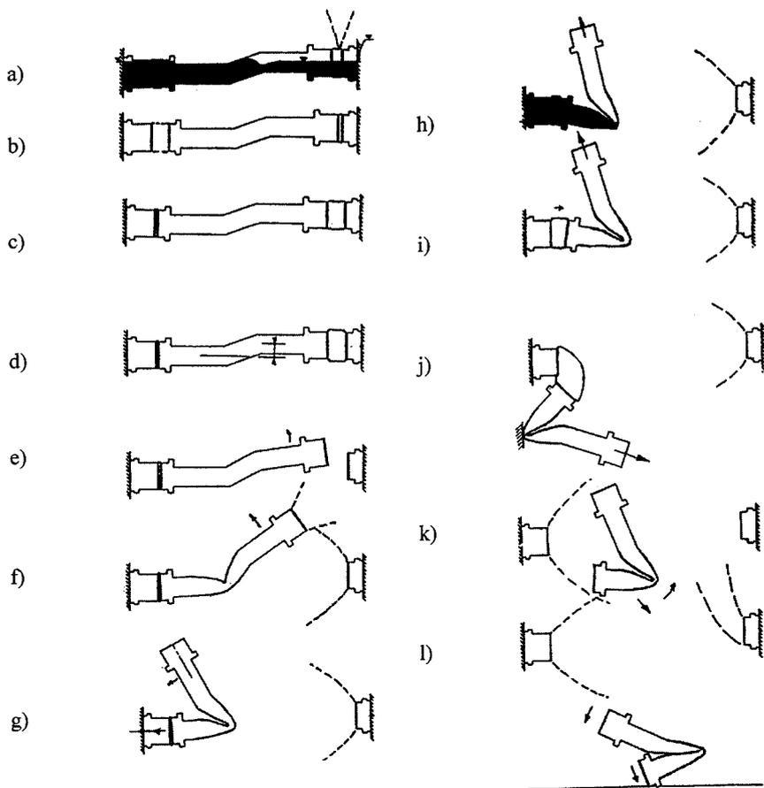
FIGURE 42.8 Successive stages of a crack-initiated two-stage bellows and pipe bridge failure.
