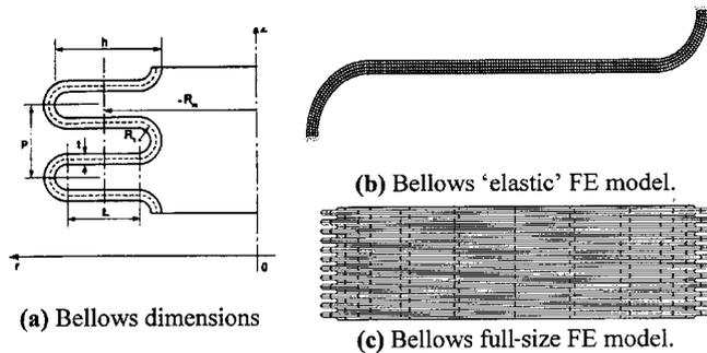
**FIGURE 42.9** Bellows dimensions and models. (Source: Venart and Tan, 2000.)
