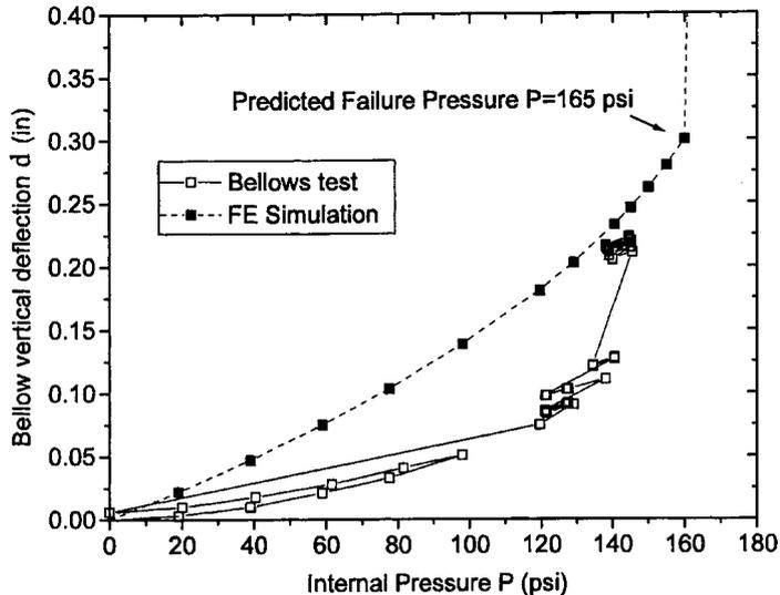
FIGURE 42.14 Bellows vertical deflection as a function of pressure; test, Batstone (1975) and FE simulation, pressure in psig, deflection in inches.
