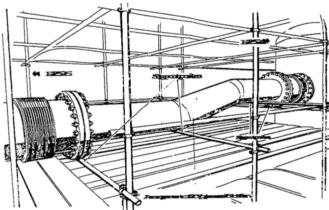
FIGURE 42.4 Reconstruction of the R5 bypass assembly showing the two 0.71-m diameter bellows and stub pipes, the 0.5-m dogleg pipe, and the support scaffolding used. (Source: Secretary of State for Employment, 1975.)
