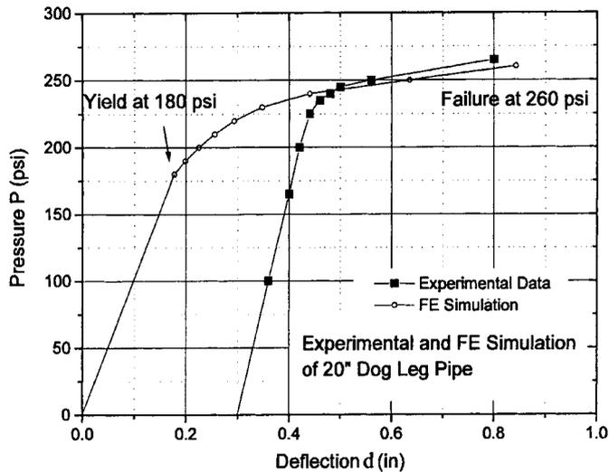
**FIGURE 42.17** Load deflection of the bypass pipe; experiment (Batstone, 1975) and FE model, pressure psig, deflection in inches. (Source: Venart and Tan, 2000.)
