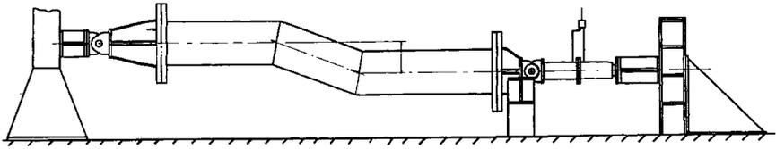
FIGURE 42.15 Bypass pipe experimental facility. (Source: Batstone, 1975.)
