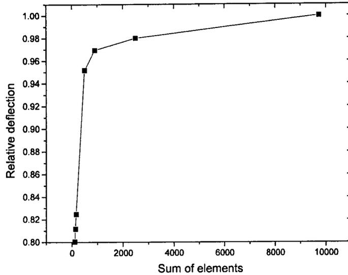
FIGURE 42.10 Total element numbers versus relative transverse deflection (stiffness).
