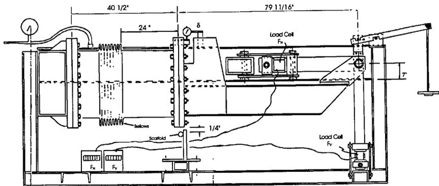
FIGURE 42.12 Bellows test facility, dimensions in inches. (Source: Batstone, 1975.)
